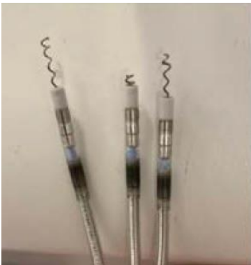
Figure 3. Complete unraveling of lead body and separation of lead helix
